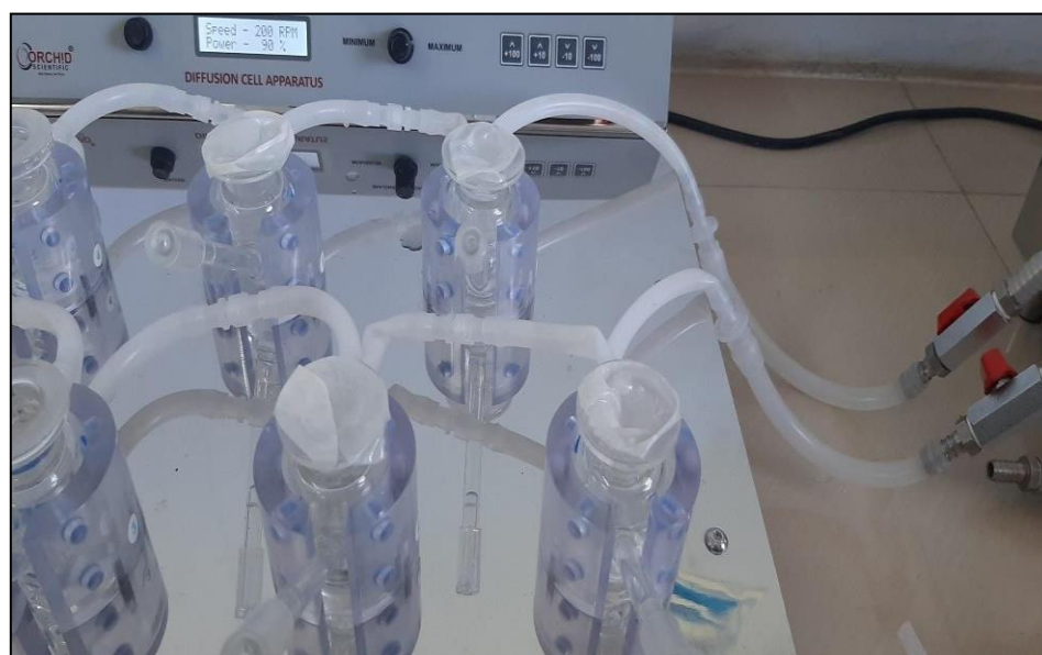
Figure No. 8: Diffusion cell apparatus along with egg shell membrane
